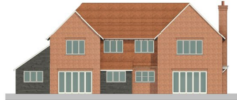
Plots 1 & 2 North Elevation (Rear) 1 : 100
